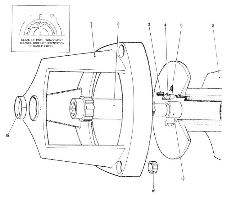
Maintenance No. 2 x 2 A Remove halliard wire from drum (6) by releasing grub screws (3) and remove winch from boat.
